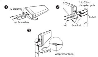
5. After narrowing down the best location for the outdoor antenna, finalize installation by using the hardware included in this kit and permanently mount it onto a mast
