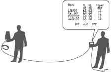
4. While pointing the antenna towards the horizon, slowly rotate around in a 360-degree circle and find the position that shows the highest maximum power output (dBm) and DL gain (dB) on the right-hand column on the LCD display **Note**: Maximum power and downlink gain for the 4K Plus & 4K Plus Pro is 10dBm/65dB and 10K Plus & 10K Plus Pro is 12dBm/68dB
