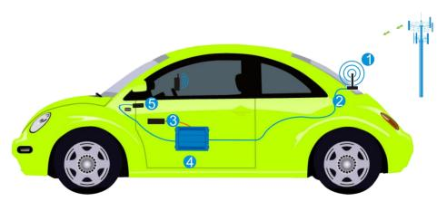
1.Magnetic Antenna 2.Cable 3.12V Car Lighter Power Supply 4.Car Booster 5.Server Antenna
