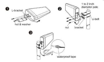
After narrowing down the best location for the outdoor antenna, finalize installation by using the hardware included in this kit and permanently mount it onto a mast
