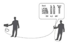
4. While pointing the antenna towards the horizon, slowly rotate around in a 360-degree circle and find the position that shows the highest maximum power output (dBm) and DL gain (dB) on the right-hand column on the LCD display
