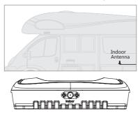
**Note**: Ensure that the front of the patch is facing in the direction where you would want signal to be distributed.
