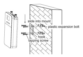
Fix the booster with the provided expansion bolt and hook. Mount the signal booster in a dry and cool area, and it shall be easily accessible for maintenance.
