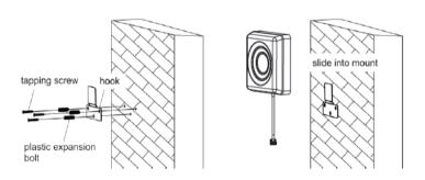
Fix the indoor antenna with the provided expansion bolt and hook.
